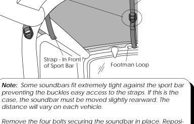
tion the soundbar rearward (check the clearance for buckle accessibility), notch out the soundbar attachment brackets accordingly - in most cases it will be less than 1/4". Reinstall the
