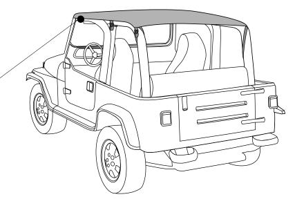
Locate Hook Strip between Sport Bar and Door Side Rail and fasten to Loop
