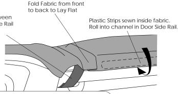
Note: When removing the Bikini, it will be easiest to remove the plastic strips by starting at the front of the plastic and pulling down and out.
