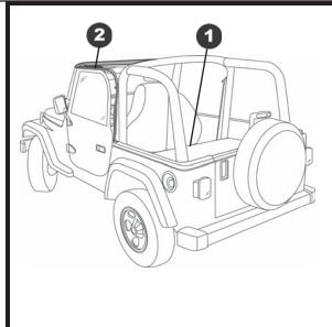
It is easier to drill holes by either slitting the carpet with a 1/2" "X" shape to access the sheet metal, or center punch through the carpet, remove the carpet and drill the necessary holes then add smaller slits in the carpet to access the holes for attachment.
