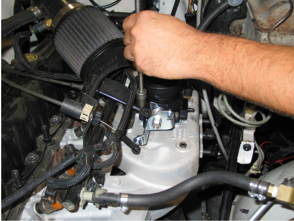
Figure 4.0 Installing and Torque the new fasteners for Throttle Body to 10in/lbs.
