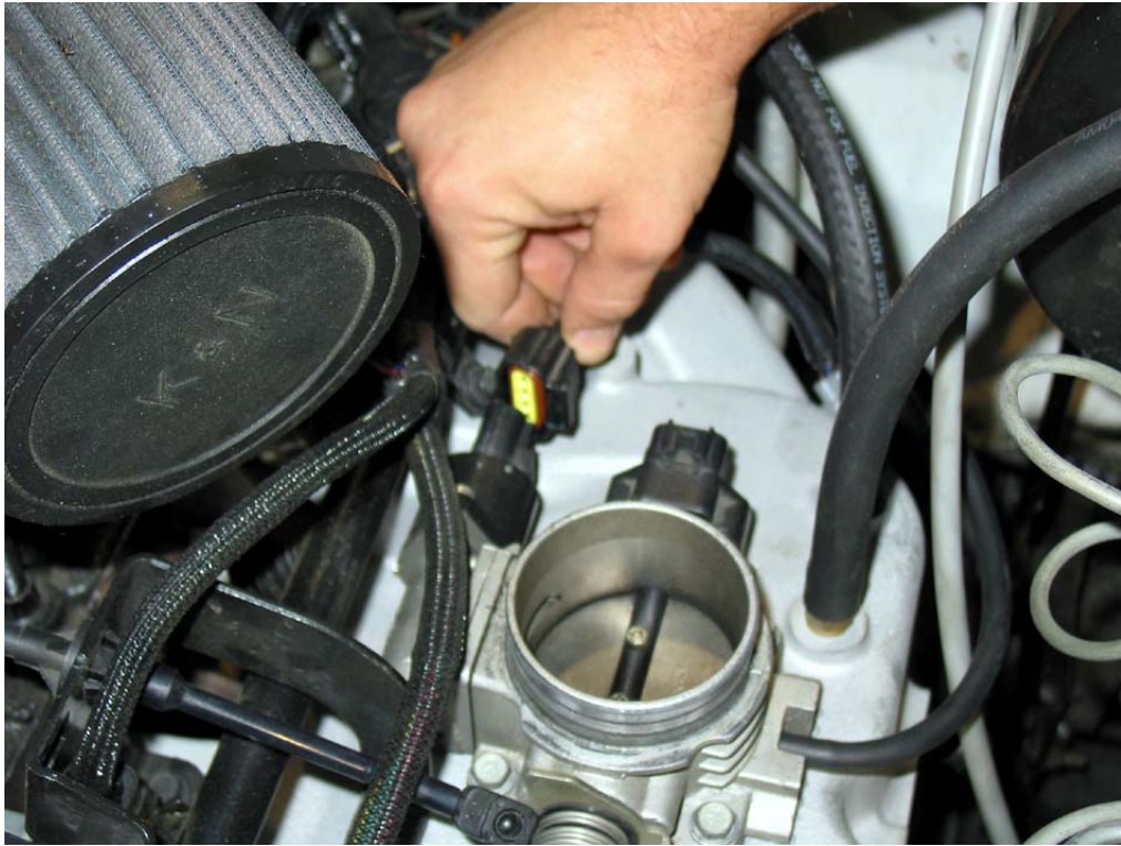
Figure 3-3 Disconnecting the IAC Motor and Throttle Position Sensor (TPS)
