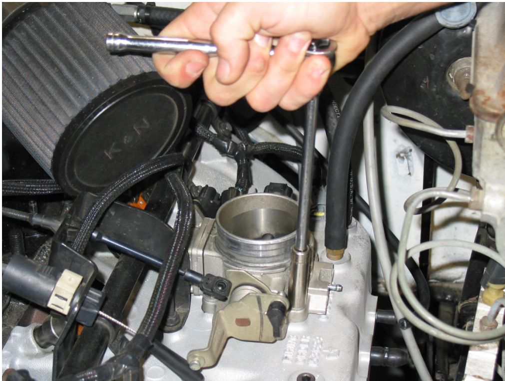
Figure 3-4 Removal of the Throttle Body and bolts.
