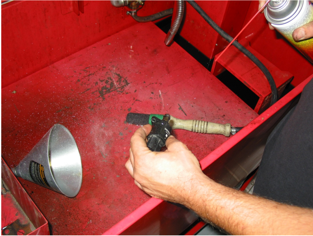
Figure 3.6 Cleaning the poppet on the Idle Air Control (IAC) Motor
