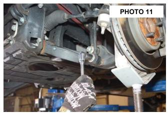
14. Remove the tie rod from the knuckle as shown using a 21mm socket/wrench. See Photo 12. Retain hardware.
