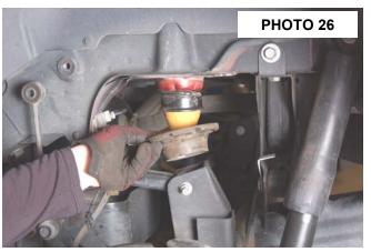
8. Remove the bump stop as shown in **Photo 27** and remove the bump stop cup from the frame using a 15mm socket. **See Photo 28.**
